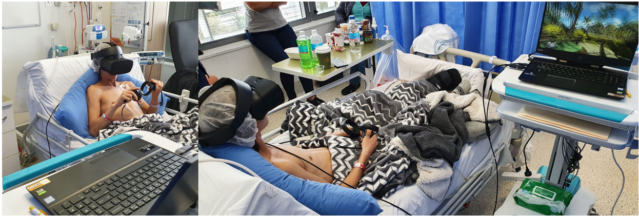
Figure 1 A readily accessible, consumer grade, high-fidelity virtual reality setup. A high-end gaming laptop allows the software to run with: high resolution graphics; low latency; and high refresh rates. The head-mounted display allows for immersive visuals and audio. Tracking sensors are integrated into the headset, removing the need for the setup to be in a fixed location. Hand controllers allow participants to interact within the virtual reality environment. This setup is easily transportable between clinical areas.
